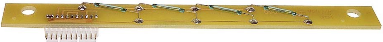
Oldest and New Version Oh Sensor (oldest version was same concept but 3 large reed switches rather than 4 small)
